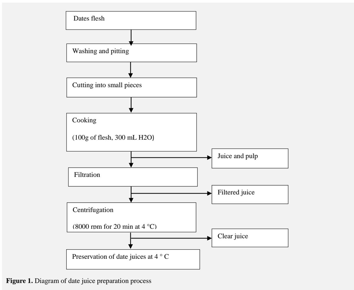
**Figure 1.** Diagram of date juice preparation process
